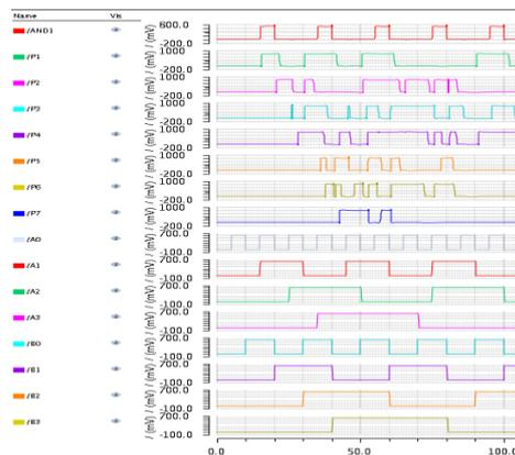
Figure 8: Braun multiplier output waveform
