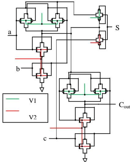
Figure 1: Full adder using double gate MOSFET
