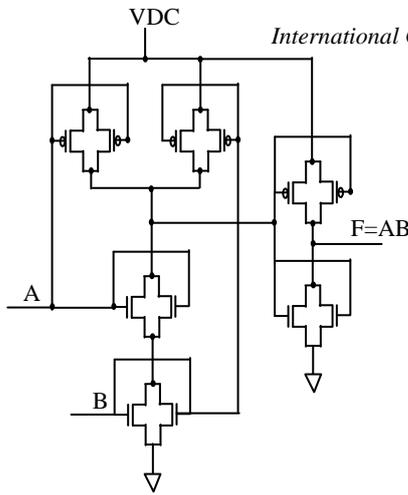
**Figure 4: AND gate using double gate MOSFET**
