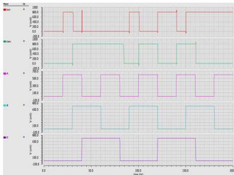
Figure 2: Output waveform of full adder
