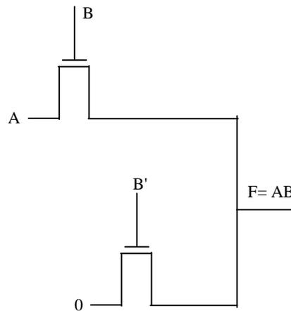
Figure 3: AND gate using pass transistor logic
