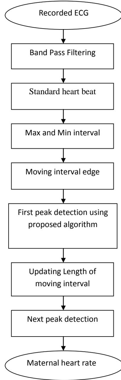
Fig 1: Block diagram of proposed algorithm
