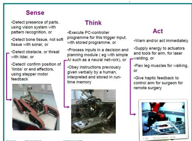
Fig. 1: Basic robotic functions and actions with examples [6] [8]
