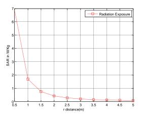
Fig 5: SAR vs. distance in human head model at frequency 925MHz
