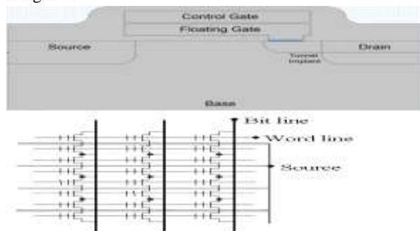
Figure 1. NOR flash array equivalent [6]
